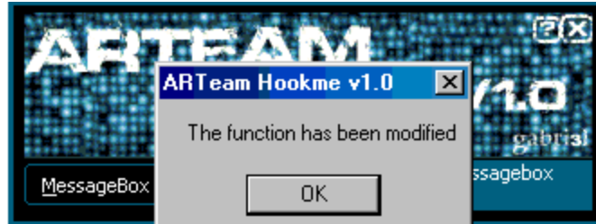
Figure 21 - Final Result of Using a DLL to Redirect API Call
